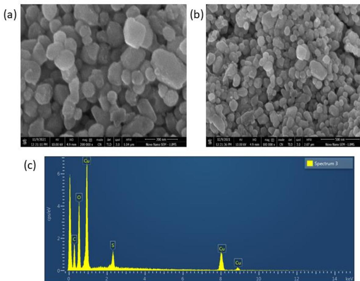
Figure 1. Characterization of synthesized copper oxide nanoparticles (CuO NPs) (a) Under 200,000X Power (200 nm) (b) Under 100,000X Power (500 nm) (c) EDX (Energy Dispersive X-Ray).
